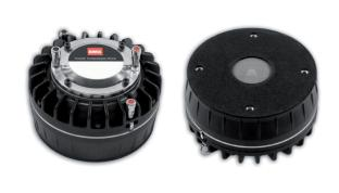
The 4595ND is a 1,5" coaxial compression driver delivering a real coherent single point wave front without hot spots with excellent phase coherence and perfect time alignment. The driver is in fact a 2-way system employing two concentric annular ring diaphragms. Each driver covers a smaller frequency range for increased power handling, high dynamic and extremely low distortion.
