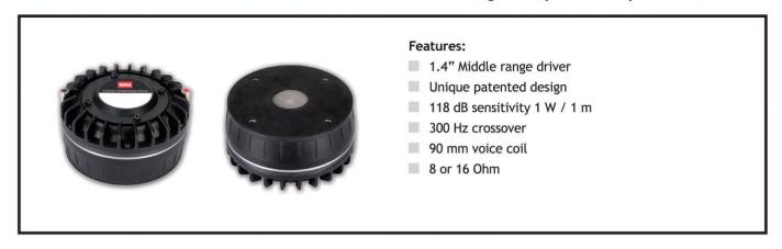
BMS 4594ND-mid is a powerful 1.4" professional compression driver that delivers outstanding sonic quality in a small package. The BMS exclusive voice coil technology employs a light weight Copper Clad Aluminium wire wound inside and outside of the Kapton™ former to improve the heat dissipation, dramatically increasing the acoustic output and reliability of the driver while minimising the power compression.
